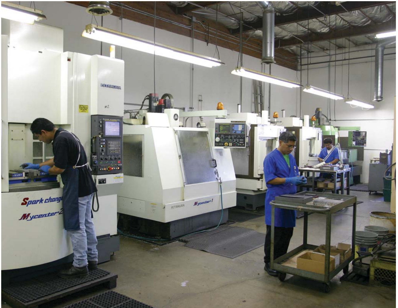
View of 4 of Conejo Industries 10 Kitamura machining centers. Operators are foreground Pedro Hernandez, machine operator, Abraham Sanchez (front right). Machines are Mycenter 2XiF Spark Changer, a Mycenter 1 and two Mycenter 0 Spark Changers (rear).
